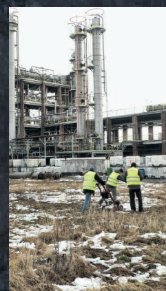
Chemical Plant Solveco – georadar studies for underground object location
