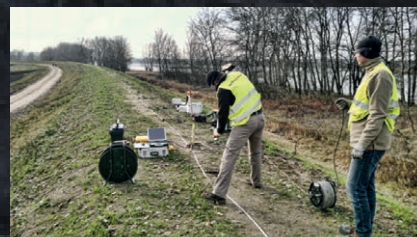
Wisla river flood embankment, Plock – seismic testing of continuity of built - in DSM barrier
