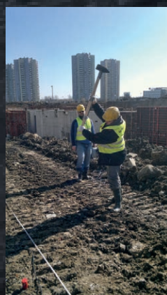
Hardcoal mine, Silesia – seismic studies for large buildings
