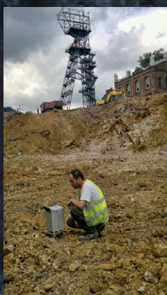
Hard mine, Katowice – gravimetric studies in the shallow exploitation area
