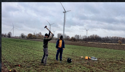
Wind farm – seismic testing for new wind turbines
