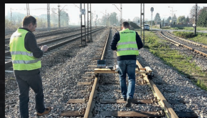
Silesian rail trial – high - resolution georadar profiling for railway line modernization
