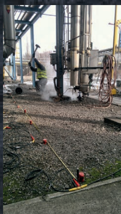
Oxygen installation AirLiquide – seismic testing in area threatened by subsidence
