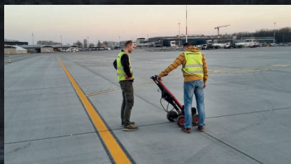
Airport Cracow Balice – georadar studies of taxiway surface and construction
