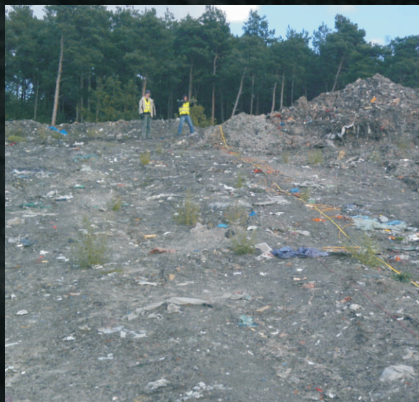
Seismic measurement on a municipal waste landfill to determine the depth range of the embankment and waste layers.
