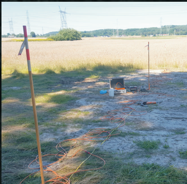
Studies of geoelectrical resistivity using ERT method.
