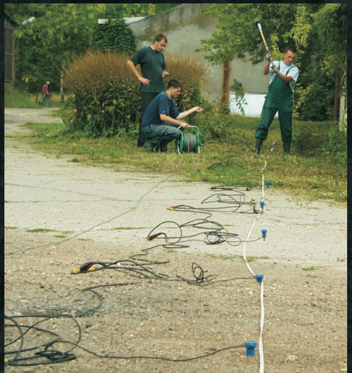
Seismic studies for geotechnical recognition before the planned housing development.
