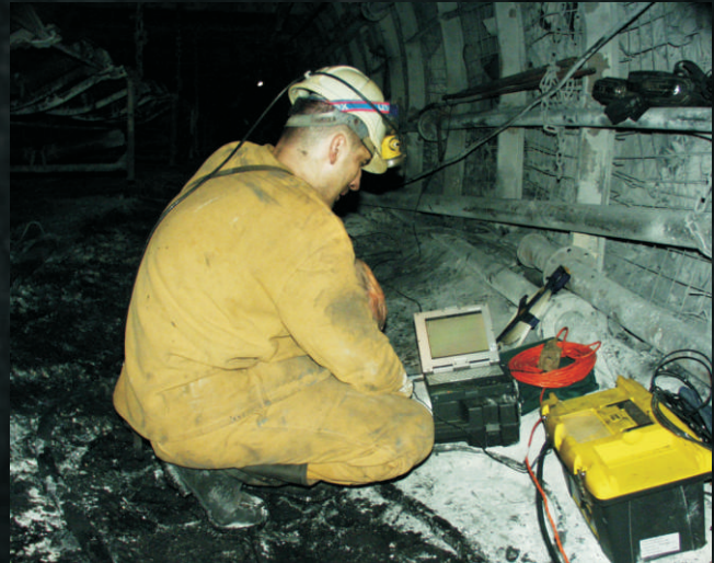
Seismic survey to assess the risk of rockburst in hardcoal mine (top).
