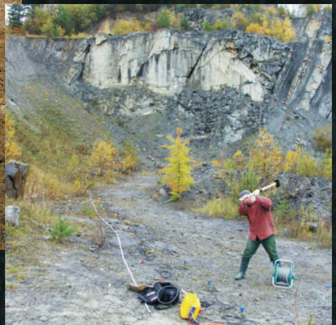
Engineering seismic surveys to determine the thickness of the weathered layer in sandstone quarry.
