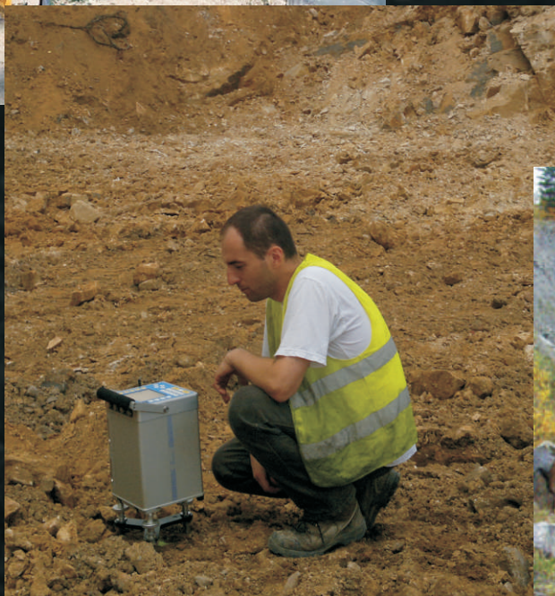
Microgravimetric survey to locate the waste-ring voids being the result of shallow mining.
