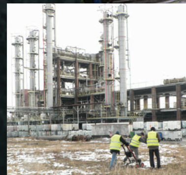
Seismic acquisition for searching underground rooms (chambers, tunnels) or their remains around the archaeological site.
