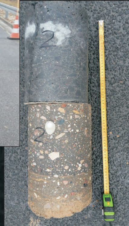
Mechanical drilling in concrete layers on highway, located in place of observed and marked cracks on surface (top) and a core of two outer layers of concrete separated by a geotextile, with a visible long vertical crack in top layer (right).
