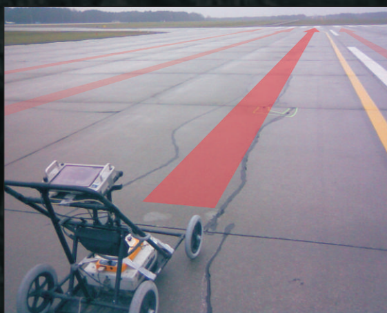
Georadar survey at airport runway.
